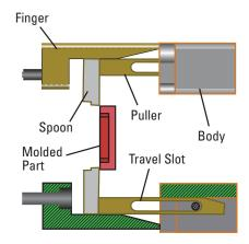
2) As the mold opens, the molded part is stuck to the core side of the mold. The Spoon, which is sandwiched between the core side and the molded part, remains in the core side of the mold during the initial mold opening movement.
