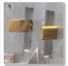
Quick Strip is actuated by the opening of the mold; reset by the closing of the mold.
