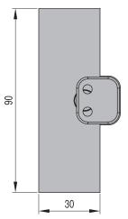
Spoon to be adjusted by moldmaker to fit mold and product contour.
