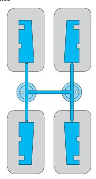
Runner Shut-Off Inserts are shown above in the open position, which allows material to flow to all cavities.
