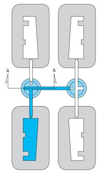
By rotating the center core of the Runner Shut-Off Insert 90° or 180° with the screwdriver end of a brass rod, material flow to one or several cavities can be shut off, as shown above.
